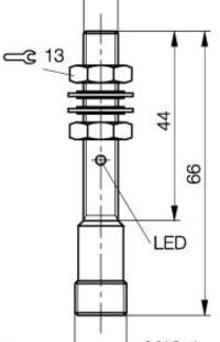
**Inductive Sensors** BES M08MH1-PSC30B-S04G M8x66 normally-open Sn=3mm quasi shielded
